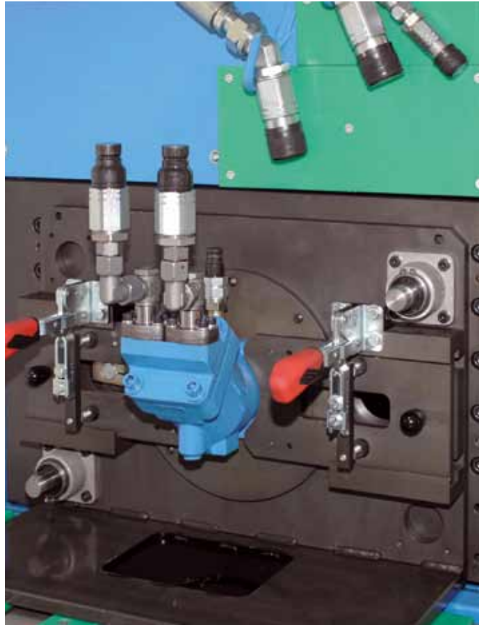
test bench for motors
